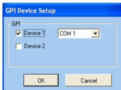
**GPI Device Setup (ALT+G)** - settings for **GPI**. ✓ **Device 1** or ✓ **Device 2** - titles and logos boxes can be assigned to the buttons of external remote control panel. Select the serial port COM (RS232) on your computer, which is connected to the external control panel;
