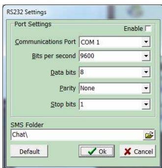
**Serial port settings** is used to get a SMS messages trough computer **Com** port.
